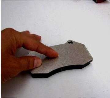
Apply the P-DEF plate and maintain a light pressure for few seconds until the glue sets.
