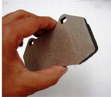
The brake pad complete with P-DEF system is ready for use.
