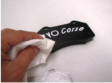
Clean up carefully the brake pad back surface
